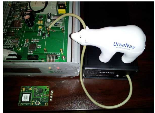
Figure 7: Modification of Frequency Data Recorder with UN-152 eLoran Timing receiver.
