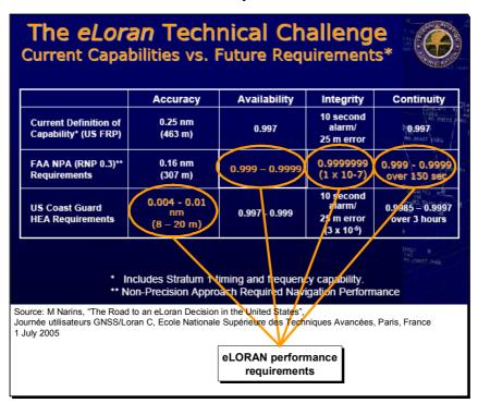
Clearly, this formidable set of requirements exceeds in respect of every parameter the performance standards of traditional LORAN-C. The modernisation of the system that has enabled this higher performance to be achieved is detailed in the set of "eLORAN actions" presented in the tables below. These may be regarded as a checklist of the improvements required to bring the US LORAN-C system up to the new eLORAN standard.
