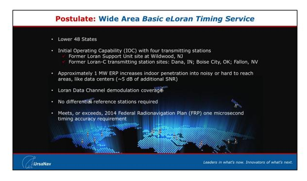
What you just saw in the demonstration was the capability of eLoran to provide accurate timing WRT UTC over a very long distance (hence, wide-area), and indoors. No differential corrections were applied.
