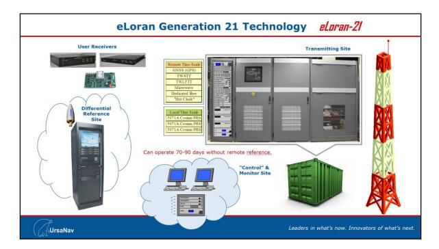
eLoran technology exists today, and is proven in operational use. The system consists of four major components: the transmitting site, the monitor & control and/or Quality of Service site, the Differential Reference site (as required), and the user receivers.
