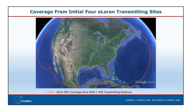
Four IOC sites are shown. Ten IOC sites are recommended, with three to the north and three to the south of the four shown. Existing Loran-C infrastructure could be repurposed for all ten sites.
