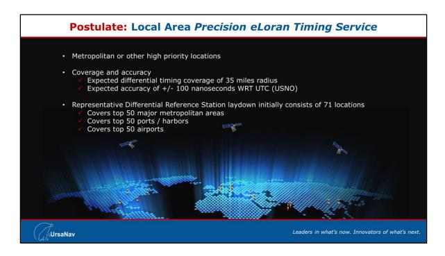
For more coverage and improved penetration into buildings, etc., additional transmitting sites are required. Additionally, PNT accuracy is greatly improved through the use of differential reference sites.
