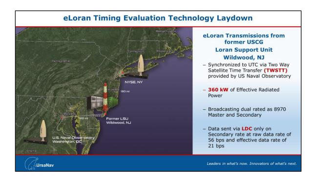
The TWSTT link between the USNO and the former LSU is provided as a UTC reference for testing. It is NOT used as a direct input to the Local Time Scale.
