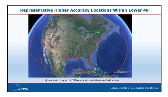
These are notional locations for differential reference station sites. Because they are key to improved accuracy within their respective coverage area, the differential reference stations have triple redundancy built in.
