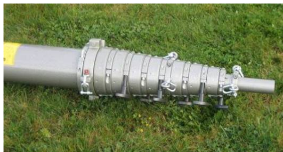
Figure 6. 21-m (70-ft) telescopic mast (retracted)
