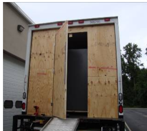
Figure 13. Transmitter truck rear false wall
