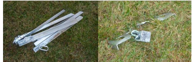
Figure 22. Antenna guy anchors and anchor supports
