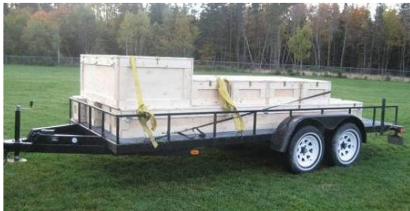
Figure 7. Antenna crate loading on a towable trailer
