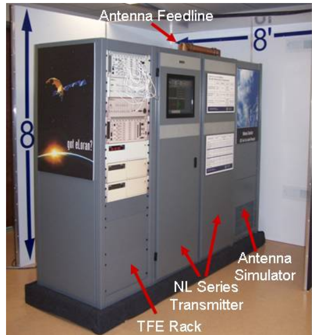
Figure 8. NL Series transmitter CONEX box mock-up
