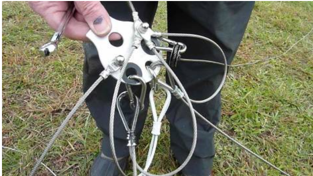
Figure 28. Antenna corner connection point
