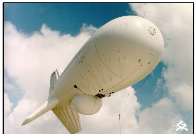
Figure 8: Aerostat Aloft Supporting an LF Antenna
