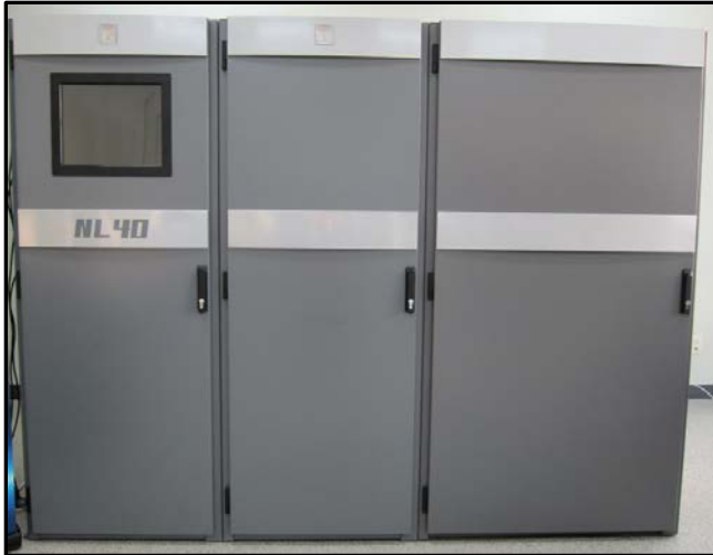
Figure 2: Nautel NL-40 High-Power LF Transmitter (Dimensions = 6 feet tall, 9.5 feet wide, 3.7 feet deep)
