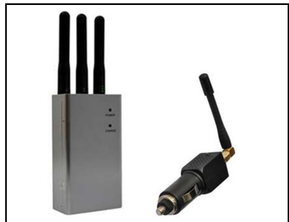
Figure 1: Low-cost GPS “Personal Privacy Devices”
